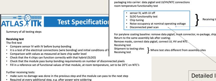
Comparison with respect to the previous test and with the first module test · Made on coated and packaged module, clean room can be relaxed to ISO9
