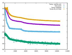
Minimal stable temperature with correct calibration at -20°C:
