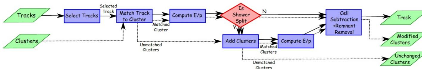
The particle flow isolation consists in a charged part, that is equivalent to the track isolation and a neutral part called ***nflowisol***, built in a similar way with the previously described calorimeter isolation but using the neutral energy flow leptons.
