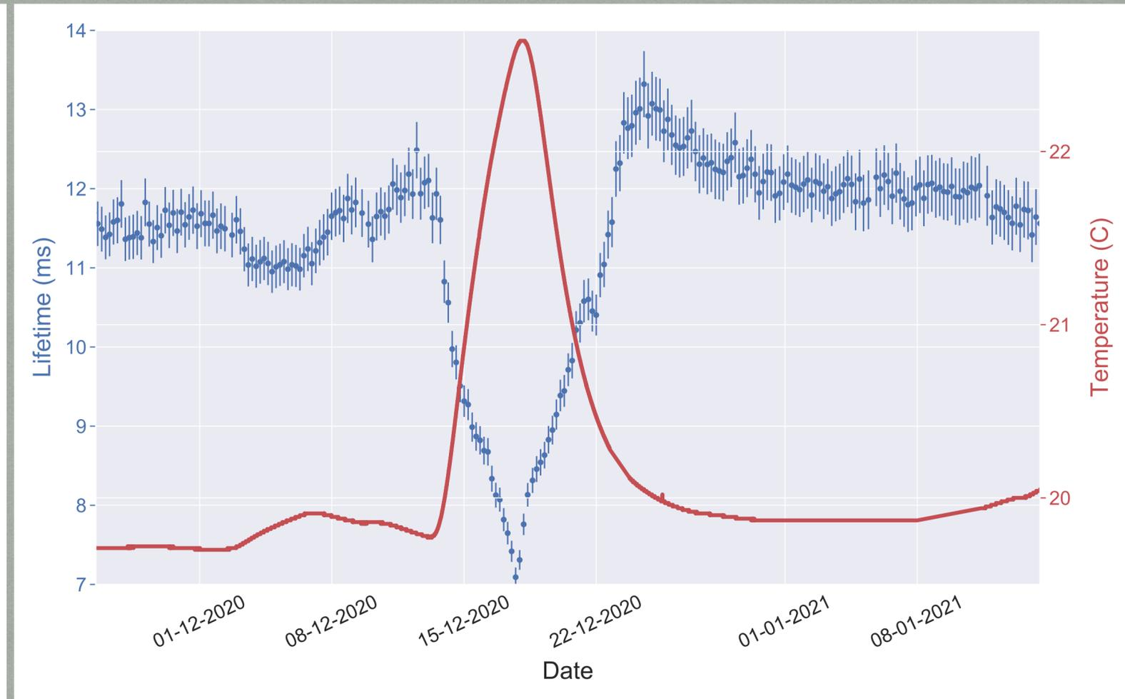
The temperature variations of the gas, driven by the variations in the laboratory conditions, affect the system behaviour.
