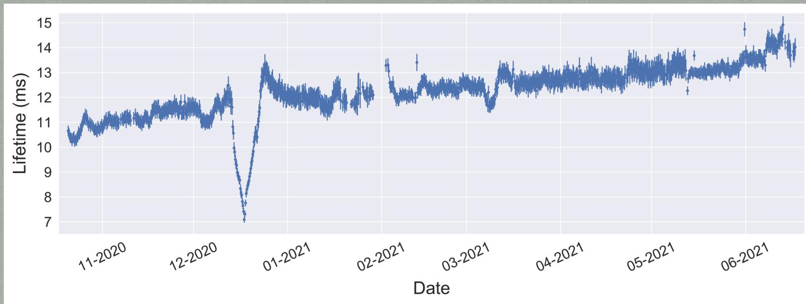
The several bumps are correlated with episodes where the temperature in the hall hosting the experiment had increased because of the air cooling system malfunctioning. In fact, it is remarkable how the variability decreased significantly after the installation of the inner castle and the radon abatement system.
