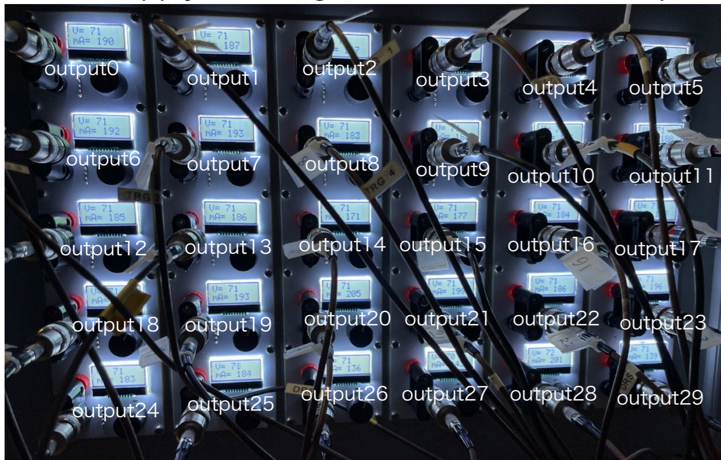
Power supply with large current : 250 mA/output, 60~80 V
