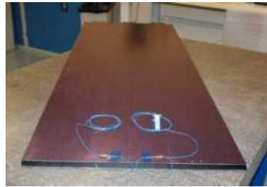
Moulding of one layer of 3 alveoli L = 2.490 m wall thick. = 0.5mm
