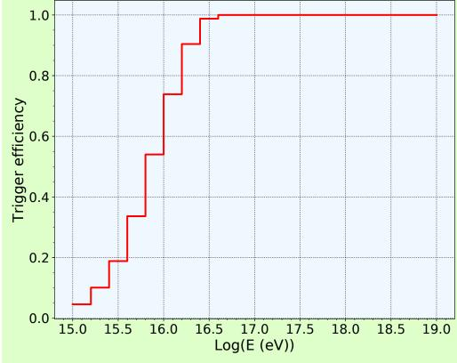
The trigger efficiency, leading to an expected event rate of order  $10^6$  per month for showers with  $0 \le \theta \le 30^\circ$ . For larger zenith angles no significant energy deposit is expected in the ice. A radio trigger is currently under investigation and expected to have a cut off at  $10^{16}$  eV.
