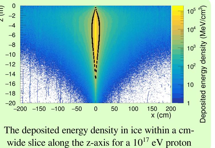
The deposited energy density in ice within a cm-wide slice along the z-axis for a 10<sup>17</sup> eV proton induced air shower. The black line indicates the area in which the plasma frequency has a value larger than 100 MHz.
