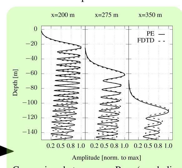
Comparison between paraProp (parabolic equation method, line) and meep (FDTD, point) at ranges of 200, 275, and 350 meters from the transmitter for a functional form of the in-ice n(z) profile for the South Pole, with an air boundary.
