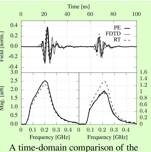
paraProp parabolic solver (thick line) and the meep FDTD solver (thin line).
