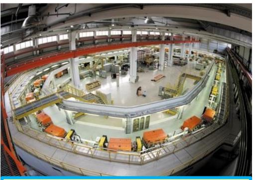
Cyclotron < 300 MeV/c Cooler-Synchrotron COSY < 3.7 GeV/c 5 · 10<sup>10</sup> stored p,d unpolarized, polarized phase space cooling internal, external target stations
