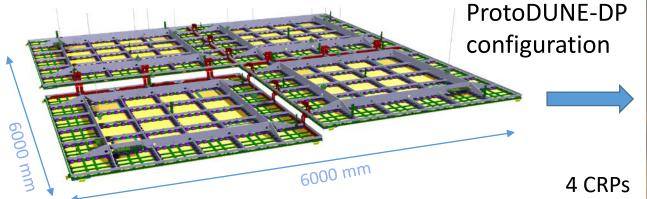
2 instrumented CRPs with 36 LEMs and 36 anodes (50x50 cm<sup>2</sup>) :
