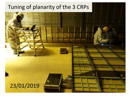
The planarity of the CRP is measured and adjusted on 50 points and 2-3 iterations.
