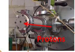
Beam line under vacuum 12 μm aluminized mylar window
