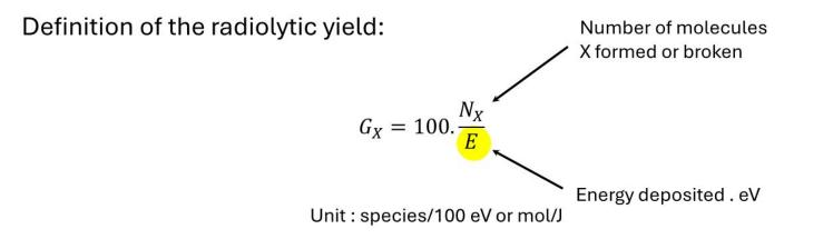
Determination of the energy deposited  $\rightarrow$  Dose measurement / Dosimetry
