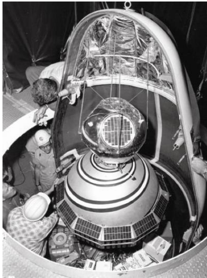
SNAP 3B in 1961 powered by 96 grams of plutonium-238 metal, aboard the Navy Transit 4A spacecraft
