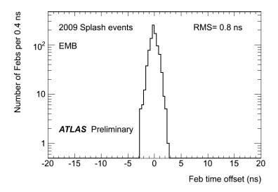
Relative timing adjusted to < 1ns (important for E resolution)
