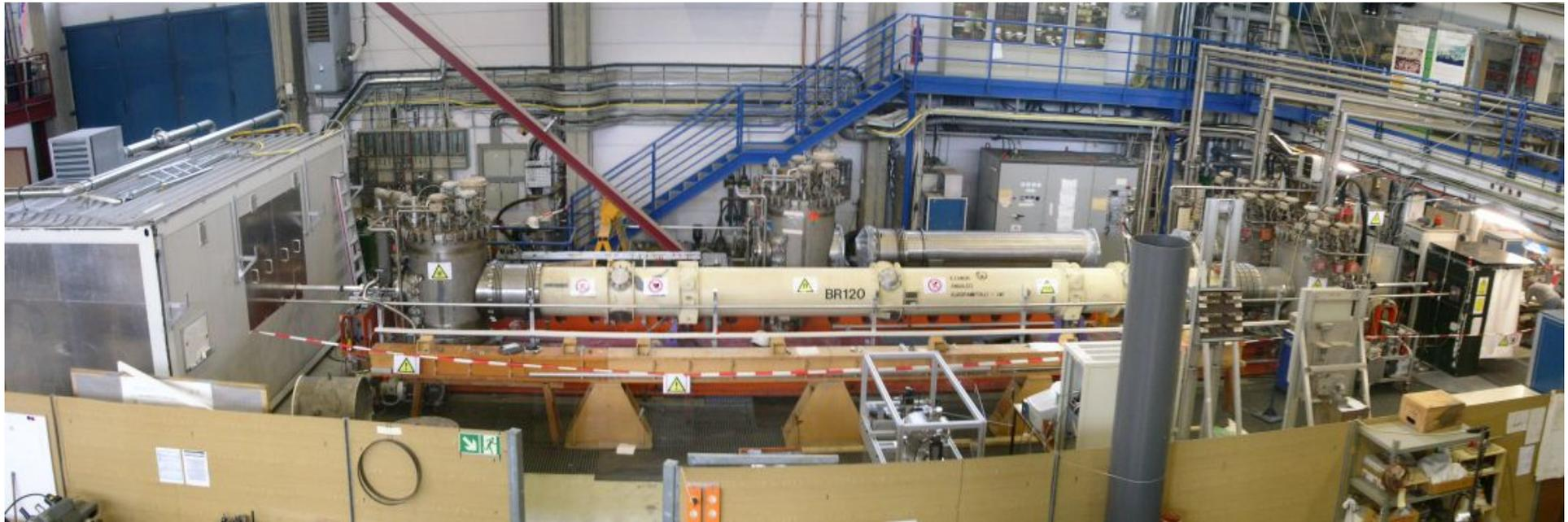
photon regeneration experiment using a HERA Dipole Magnet
