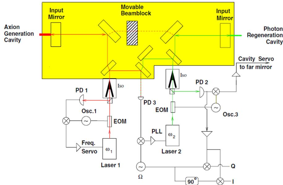
“Detailed design of a resonantly-enhanced axion-photon regeneration experiment”
