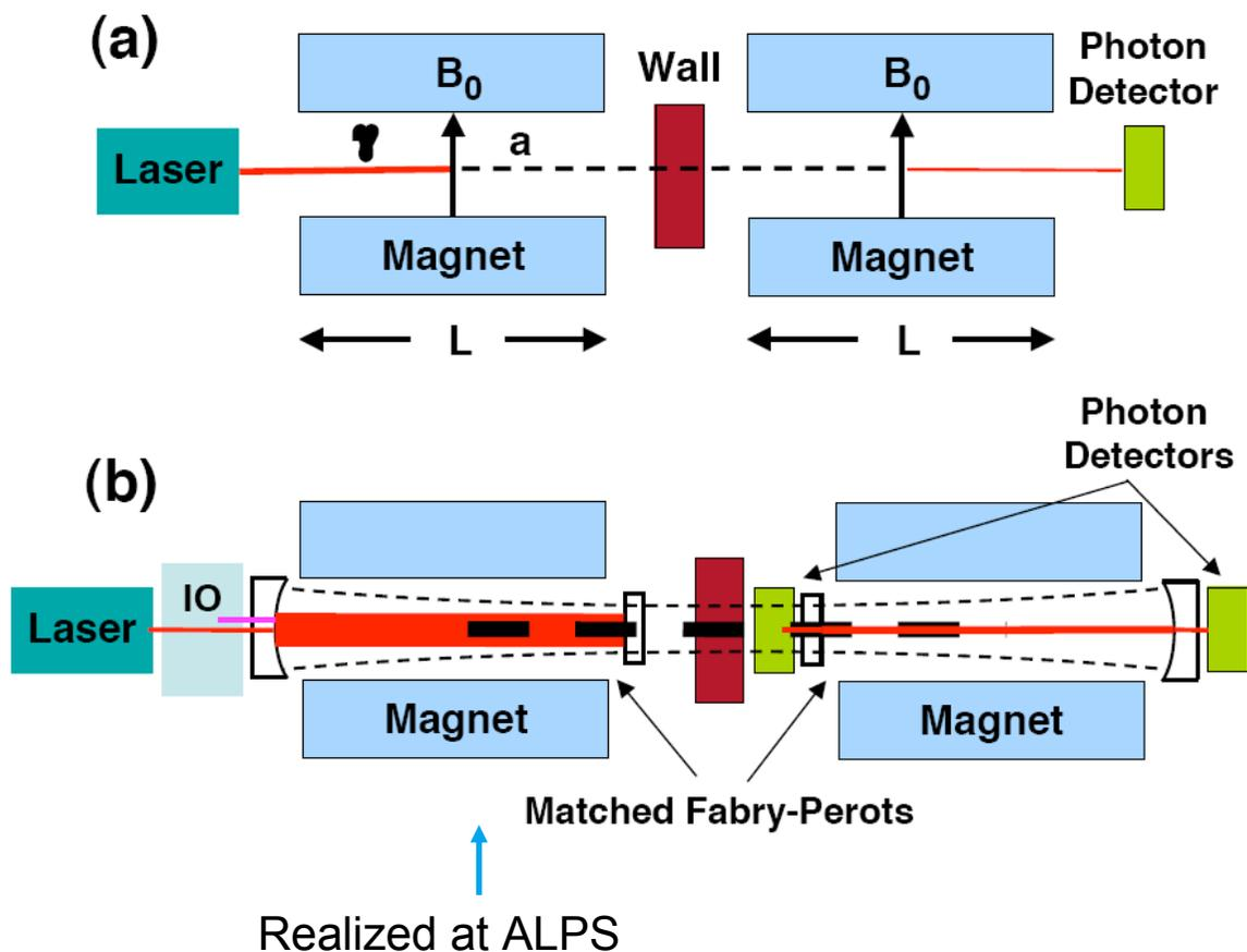
Implementation of a second cavity in the regeneration part of the experiment to enhance the conversion probability  $WISP \rightarrow \text{photon}$
