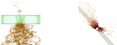
Microscopic simulation of electron avalanches in a GEM (left) and around a wire (right).
