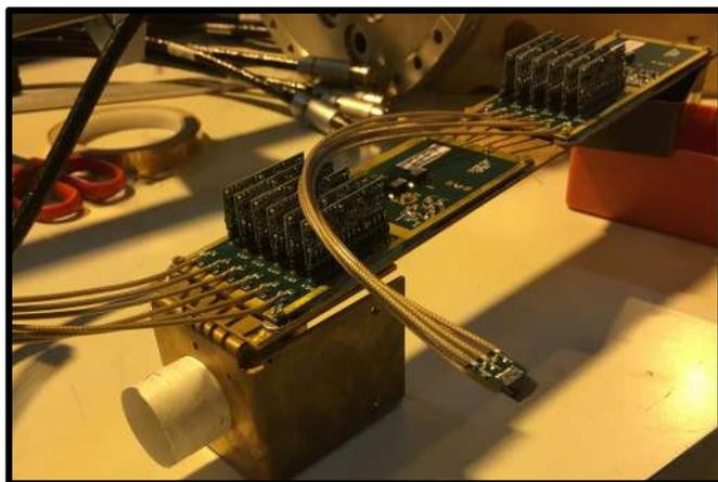
*Plastic scintillator mounted on its cube copper support*
