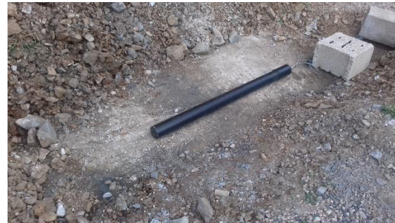
Installation of the surface magnetometer
