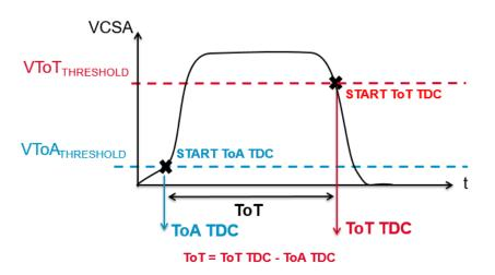
Saturation regime: 12-bit TDC Time-over-Threshold (ToT) with a 50 ps binning up to 200 ns
