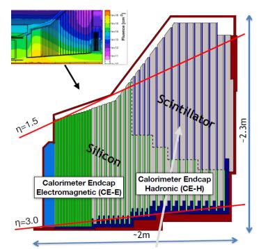
Hexagonal **silicon sensor** based modules in CE-E and high radiation regions of CE-H. **Scintillating tiles** with on-tile SiPM readout in low-radiation regions of the CE-H.
