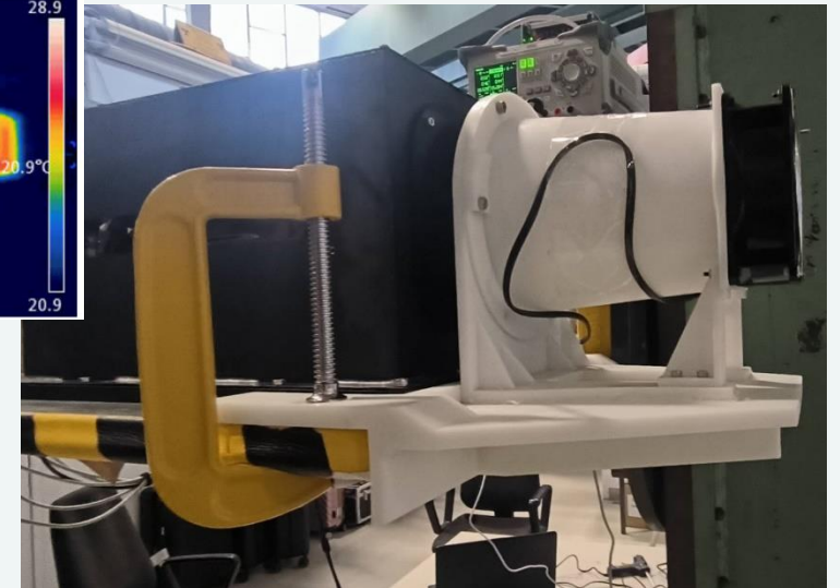
Air cooling test setup
