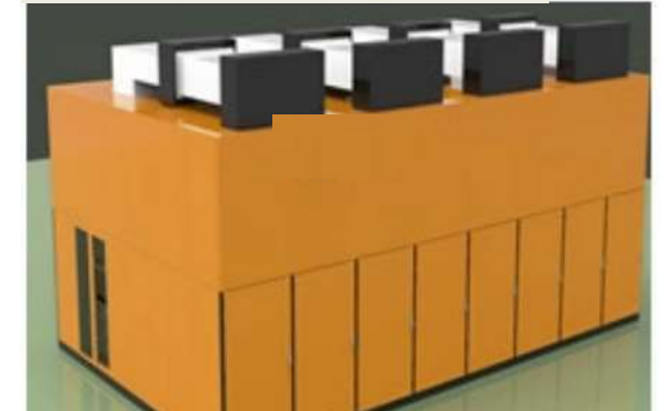
Klystron No. 3 (MBI) Efficiency 80.5% (under fabrication)
