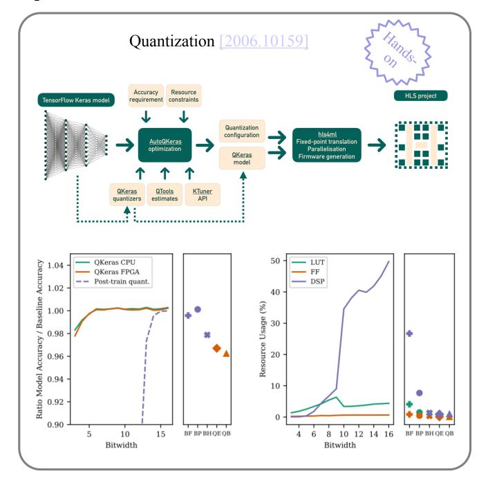
Model inference can be accelerated by reducing the number and size of operations.
