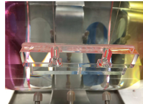
Last stage of suspension made of silicon fibers
