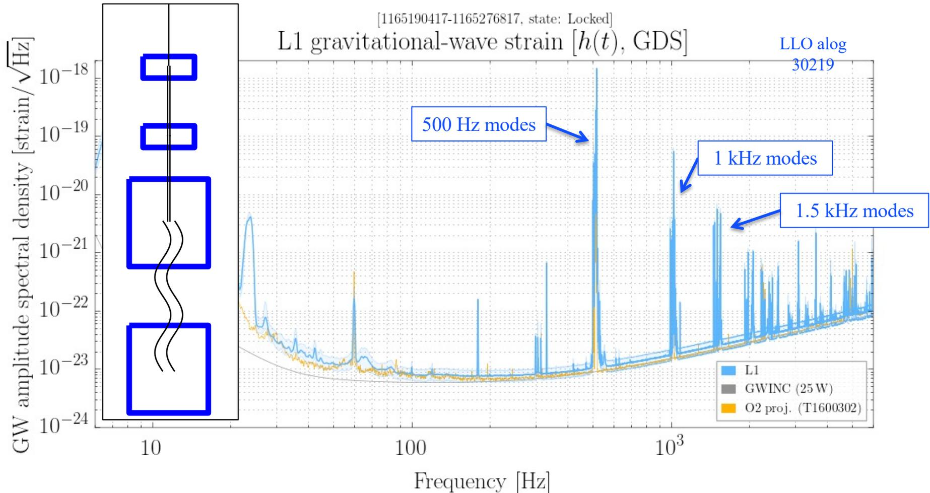
Very high Q ( $\sim 1$  billion) silica fiber violin modes at 500 Hz and higher harmonics, excited by thermal noise
