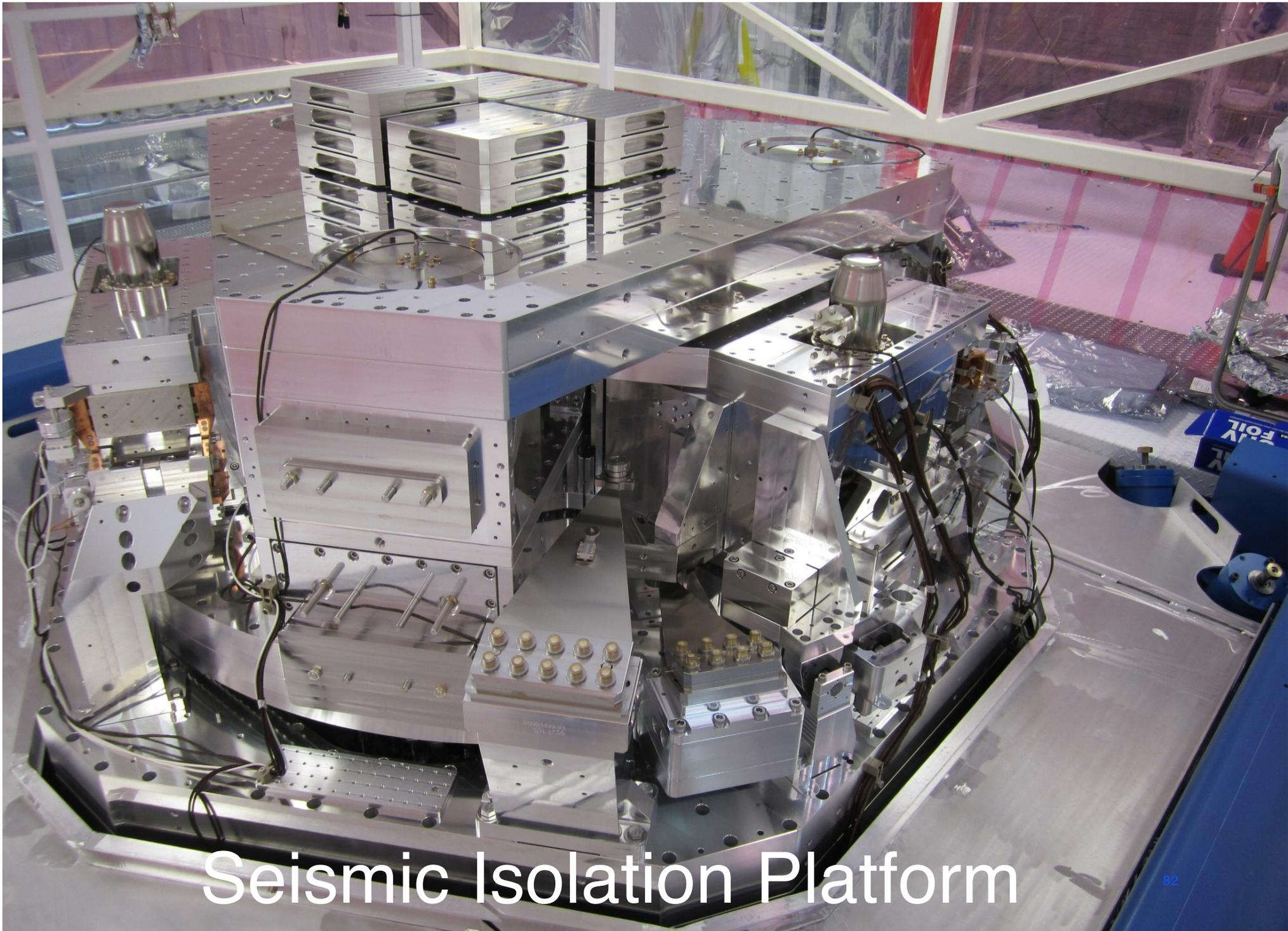
Seismic Isolation Platform
