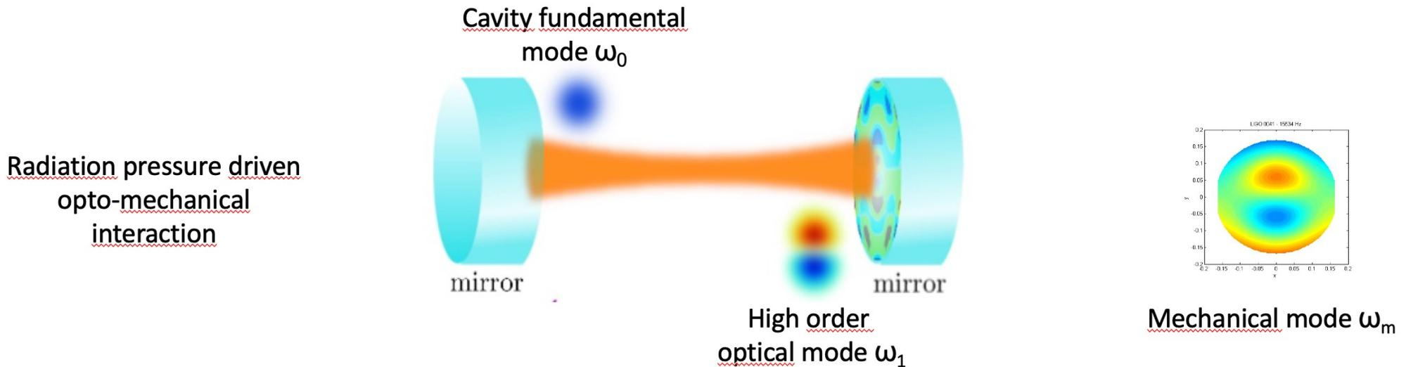
Thermally excited acoustic mode scatters TEM<sub>00</sub> mode → sidebands  $\omega_0 \pm \omega_m$
