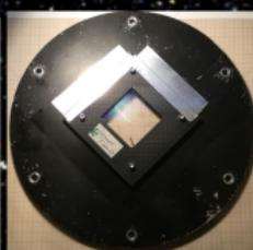
Disperser: phase hologram (150 lines/mm)
