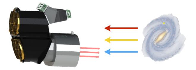
Spectra obtained by stepping sources over the FOV in multiple images: <u>no moving parts</u>
