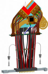
wire bonding and HV/LV/data cable attachment
