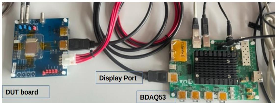
Setup for BDAQ53 Test – developed by Bonn
