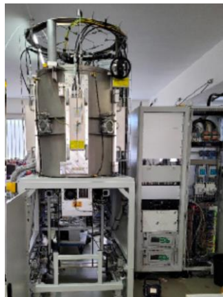
DLC Magnetron Sputtering machine co-funded by INFN-CSN1
