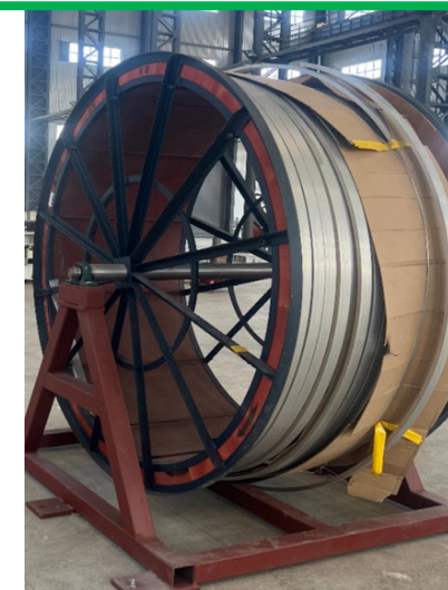
Long Dummy cable (22*56mm 2 )
