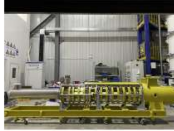
Klystron No. 2 Efficiency 77% (2021)
