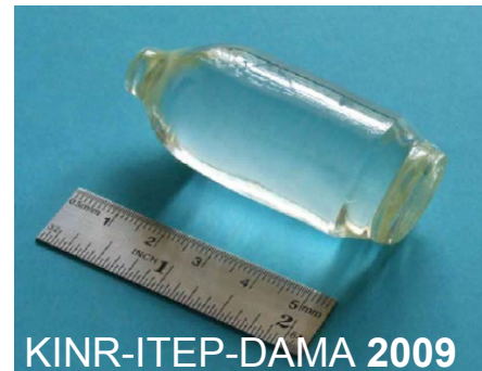
^{106}\text{CdWO}_4 (0.22 kg, 66.4% ^{106}\text{Cd} ) Nucl. Instrum. Meth. A 615 (2010) 301
