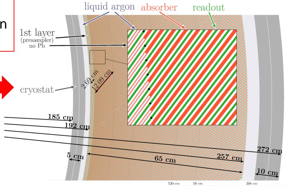
Much finer lateral and longitudinal granularity than ATLAS (x10)
