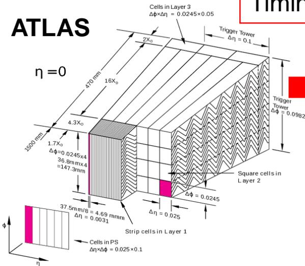
Absorber plates inclined by 50° w.r.t. radial direction
