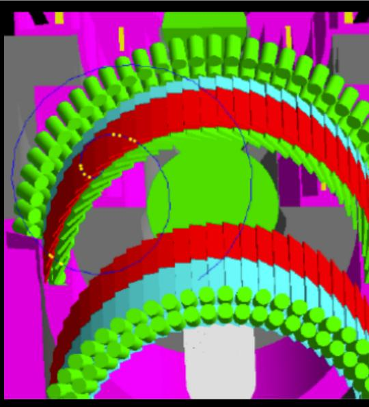
2-rings of ultra fast scintillators 64 segments, 33/36 x 1 x 1 cm3 read by optical fibres and SiPMs
