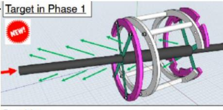
Graphite Diameter: 26 mm and 40 mm, Length: 700 mm
