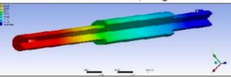
FEM simulation is completed. Max. temp. 245 degC.
