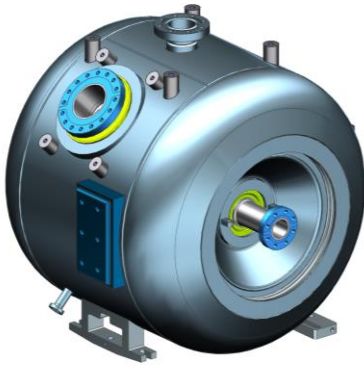
3D view of the jointly designed SSR2 Spoke resonator
