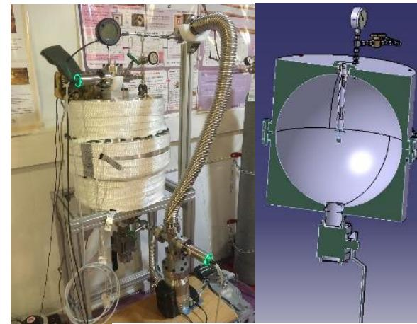
② 50 kg enriched Xenon Cu detector, 40 bars, 37 cm radius
