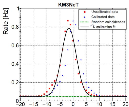
Coincidences between PMTs on a DOM allow time, efficiency and transit time spread calibration
