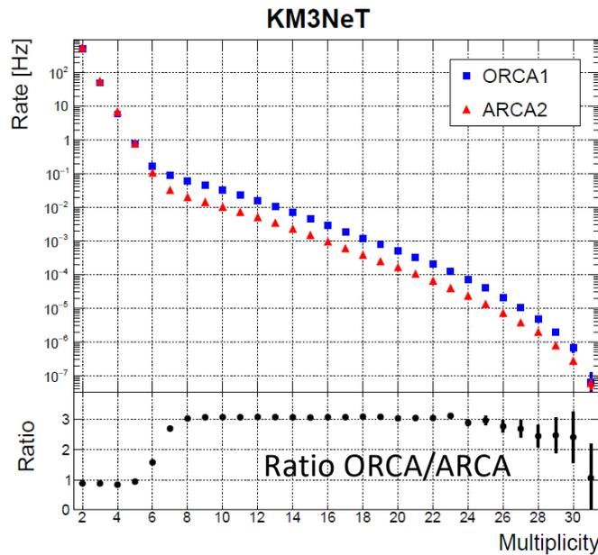
Above a multiplicity of 8 PMTs, rate is dominated by atmospheric muons
