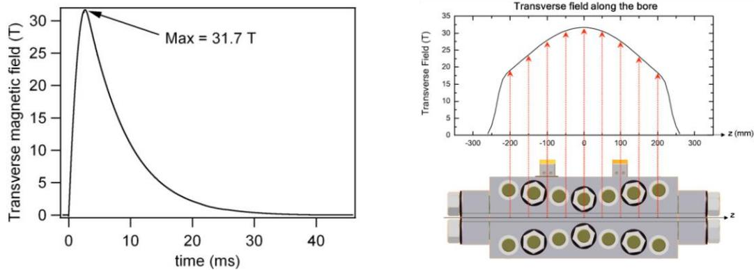
**Fig. 2.** XXL-Coil Left: magnetic field pulse of the XXL-Coil as a function of time. Right: measured magnetic field profile along the longitudinal axis.
