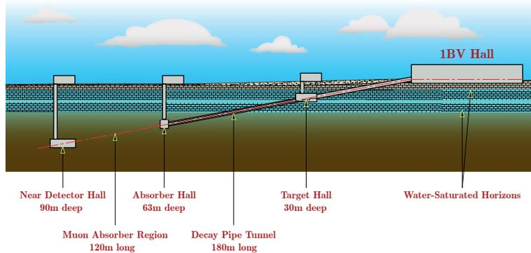
Figure 2: Elevation view of the proposed neutrino beamline (the baseline design).
