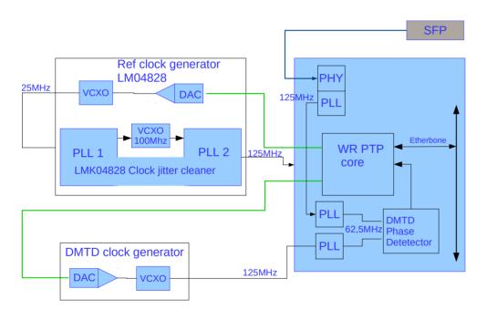
The WhiteRabbit IDROGEN hardware is base on CERN open hardware with Enhancements
