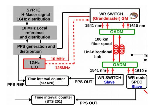
For the test we use the test system developed by the SYRTE for timing distribution measurement.
