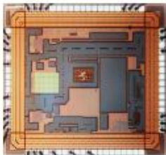
SQMUX8 2x4 TDM .2 nV/VHz 5 MHz 4K
