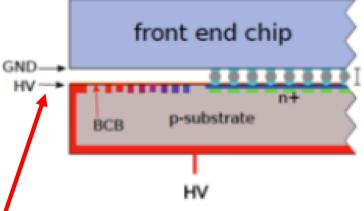
This huge voltage difference generates a strong field across the few  $\mu m$  of sensor-chip separation and can give rise to sparks
