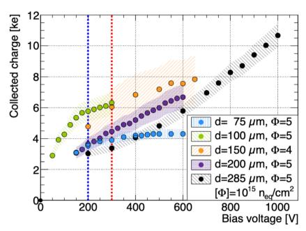
Even at very high fluence (for planar pixels), thin sensor can guarantee an excellent hit reconstruction efficiency
