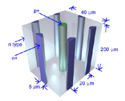
Here the electrodes are columns passing from one face to the other
