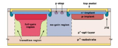
A few techniques are available to avoid this limitation: one is the use of Inverted-LGADS (I-LGADs) where the multiplication layer is on the opposite face
