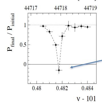
Resonant depolarization is produced by exciting the beam with an oscillating magnetic field generated by a vertical kicker magnet (field in the horizontal plane)
