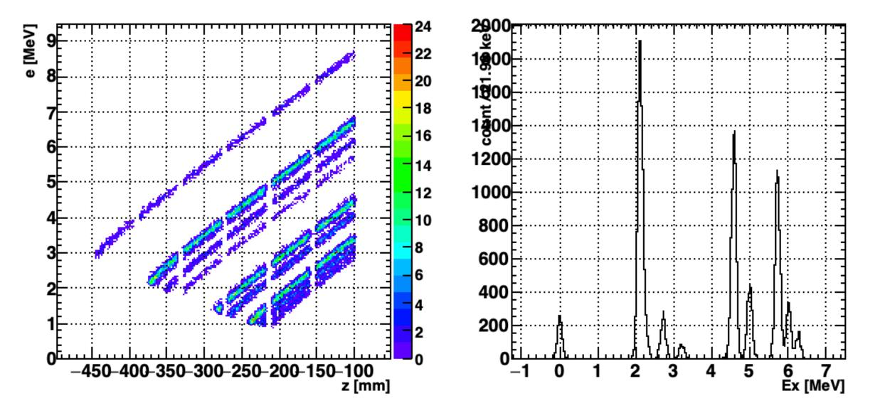
$$E_{lab} = E_{cm} - \frac{1}{2}mV_{cm}^2 + \left(\frac{mV_{cm}}{T_{cyc}}\right)z$$
