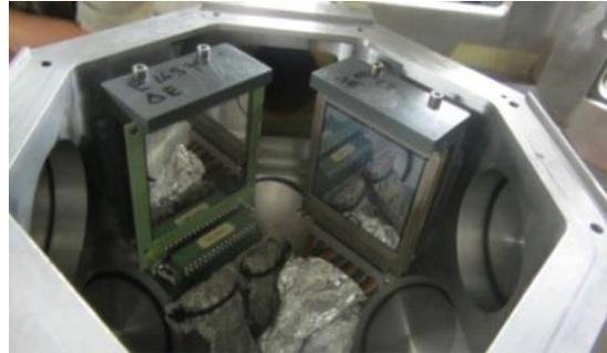
300MeV  $^{86}\text{Kr}$ , CD targets. HPGe +  $\text{LaBr}_3(\text{Ce})$  + Silicon
