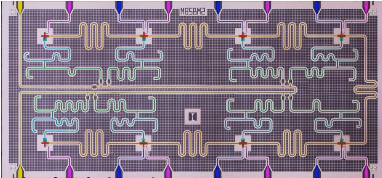
*Figure 3: False-coloured image of an 8-qubit superconducting quantum processor fabricated at ETH Zurich. All eight qubits (red) are measured using a common readout line (yellow), by coupling each qubit (red) to a pair of readout resonator (cyan) and Purcell filter (green). Qubit control is enabled by individual charge lines (purple) and flux lines (blue). Coupling between nearest neighbour qubits is mediated by bus resonators (orange).*
