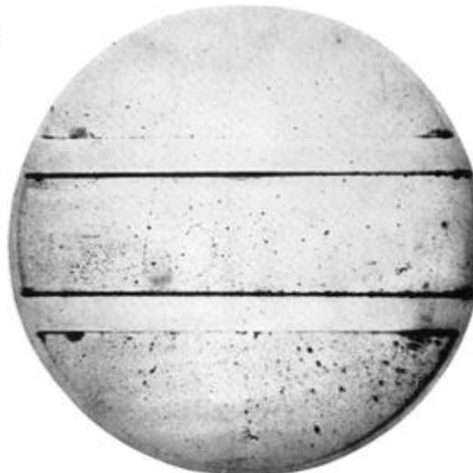
FIG. 1. A 63 million volt positron ( $H_D = 2.1 \times 10^5$  gauss-cm) passing through a 6 mm lead plate and emerging as a 23 million volt positron ( $H_D = 7.5 \times 10^4$  gauss-cm). The length of this latter path is at least ten times greater than the possible length of a proton path of this curvature.
