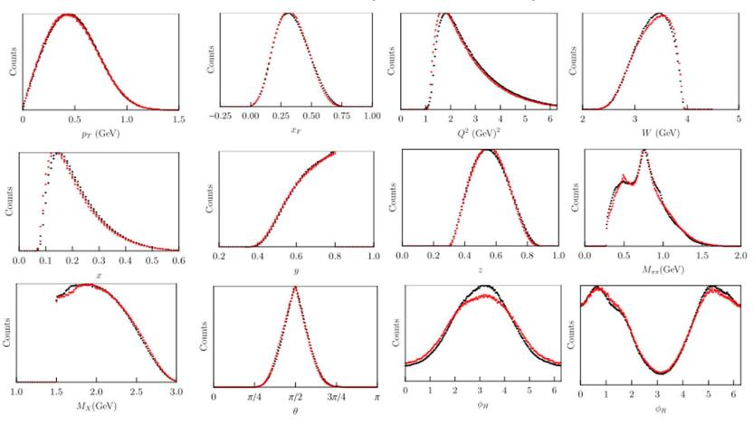
CLAS12 MC, based on the PEPSI(LEPTO) simulation with <u>most parameters "default"</u> is in a good agreement with CLAS12 measurements for all relevant distributions
