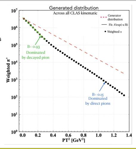
By combining the directly produced pions and the decayed pions, two Gaussian slopes are effectively generated even if we started with one single gaussian
