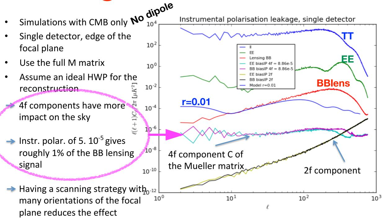
Combining several detectors at different locations of the focal plane reduces the effect since it is observed with different phases
