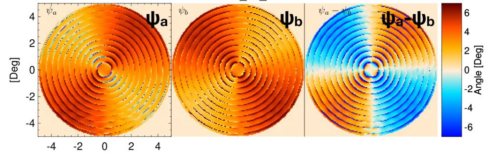
GRASP simulation for 100GHz detector @112GHz (higher bandpass edge)
