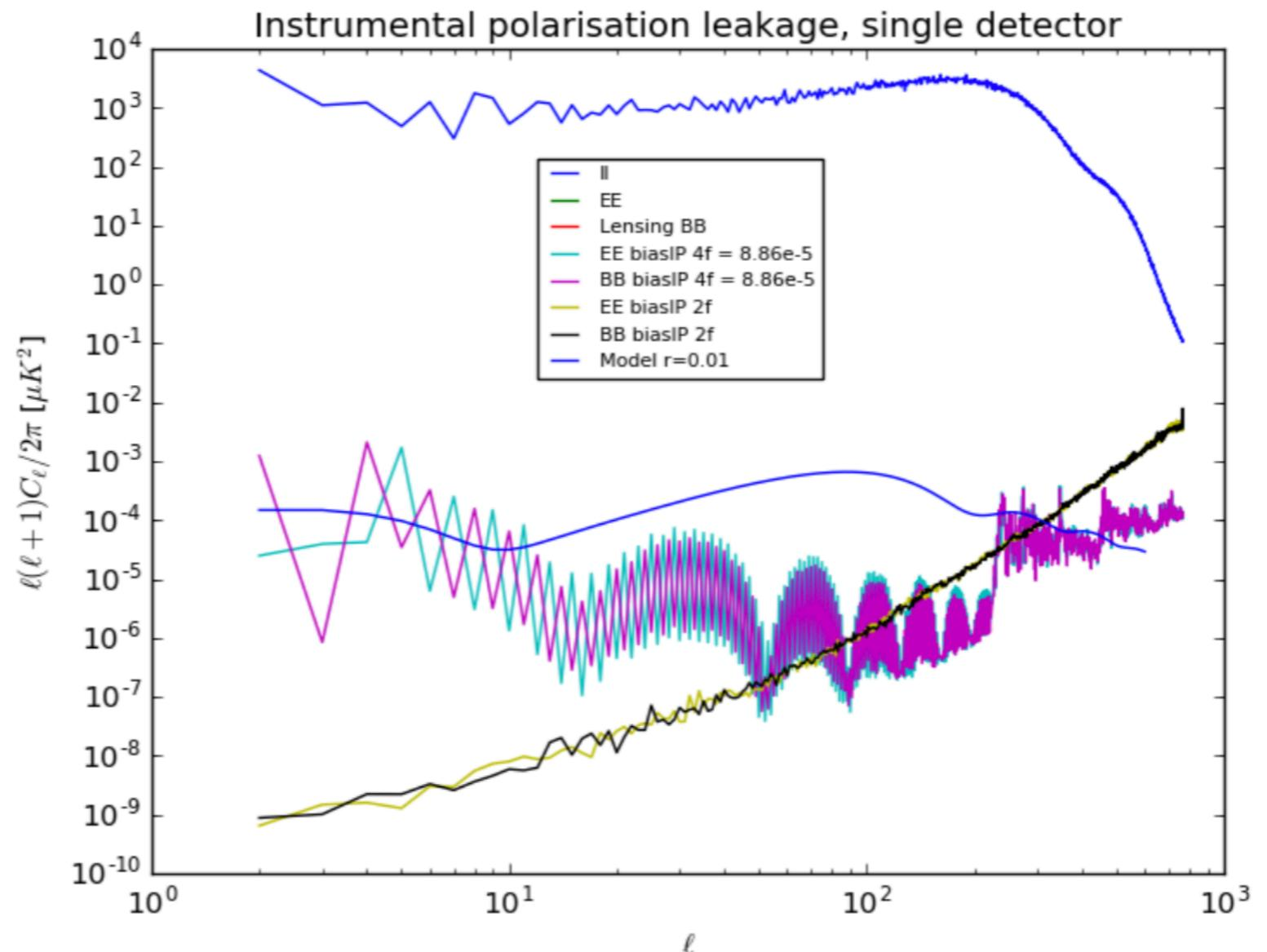
The leakage on maps can be predicted analytically by propagating the expression of the IP through the map-making equations
