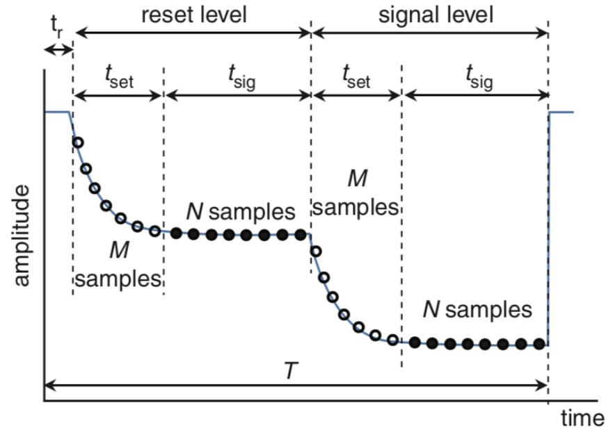
**Fig. 1** *Timing diagram of CCD output signal*
