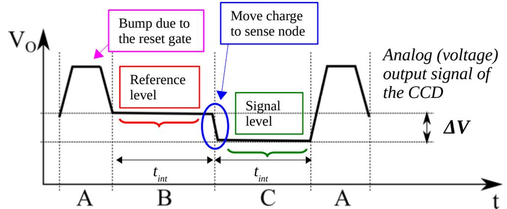
Skipper technique allows for a Non-Destructive Multiple pixel charge measurement (NDCM) which results the electronic noise to follow the  $1/\sqrt{\text{NDCM}}$  ( $\rightarrow$  A. Matalon talk)
