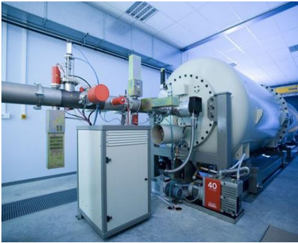
Microbeam line connected to a particle accelerator
